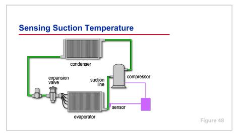
In a direct-expansion (DX) application, where the refrigerant in the evaporator is cooling air, frost protection can be accomplished in a number of ways. As mentioned, if the surface temperature of the coil gets too cold, the moisture that condenses out of the air can form frost on the surface of the coil. This "coil frosting" is detrimental to system performance and compressor reliability.
